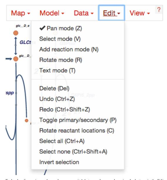
Escher has five major modes, and you can switch between those modes using the buttons in the Edit menu, or using the buttons in the *button bar* on the left of the screen.
